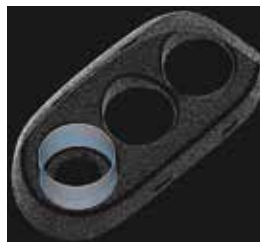
Easy reconstruct of a surface by pasting a shape on the segmented point clouds
