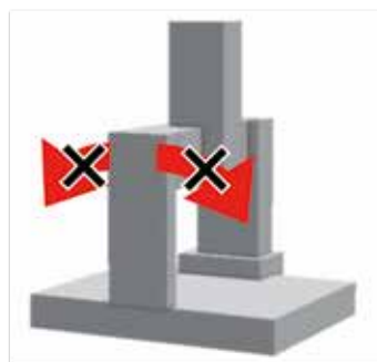
Reduction in runout in the pitching direction
