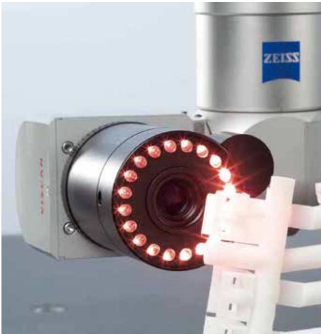
Manual setting of split light and brightness. These settings are also applied to automatic measurement.
