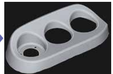
Surface connection to create a 3D CAD model
